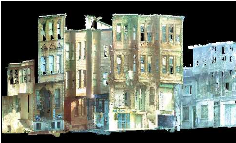
Figure 3: Street silhouette acquired via laser scanning. (This image is in sheer scale and level, and it can be brought to any desired scale.), Istanbul Fatih, Süleymaniye, IMP, Bimta A. .
