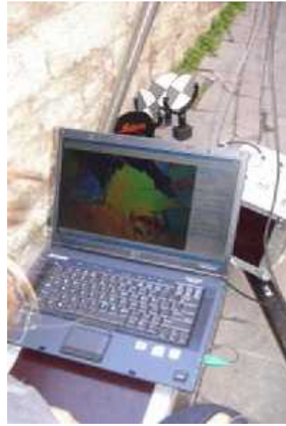
Figure 2: Data control and data transfer (Data is observed on the monitor, the frequency is determined, if scanning frequency is inadequate, a scanning with more frequent intervals is conducted –considering the lengthy duration, and a more detailed image of the facade of the building is acquired.)
