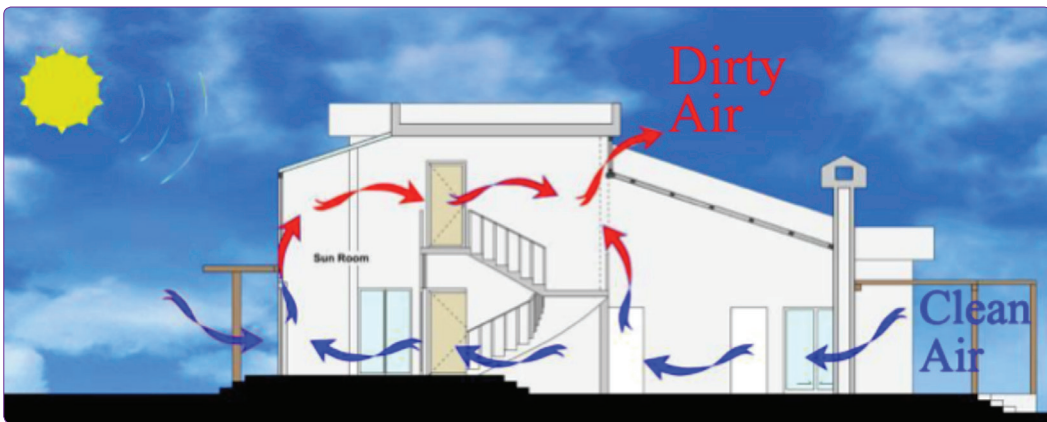
Figure 2. Section diagram of natural ventilation of a test group student (Berkey Firat).
